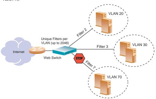
Figure 7-4 VLAN-based Filtering
